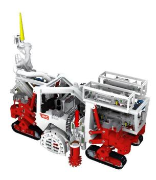
Arctic Canadian Diamond Company and IHC Mining's Underwater Mining Crawler for the Underwater Remote Mining System. The crawler will help recover diamond-bearing kimberlite ore from deep open pits at the Ekati Diamond Mine, in the Northwest Territories of Canada.
